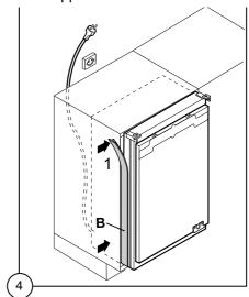
Screw appliance into place and retain the cabinet with screws (I) through the securing brackets into the worktop or adjacent woodwork as necessary.
